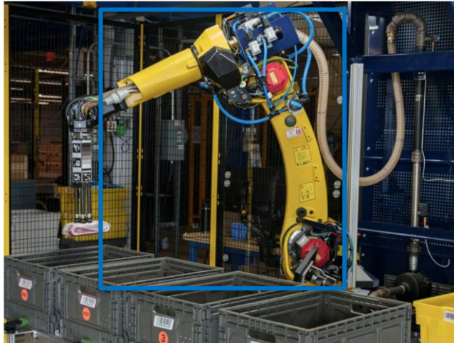
Sparrow, Amazon's latest warehouse robot, leverages computer vision and artificial intelligence to recognise and handle millions of items
